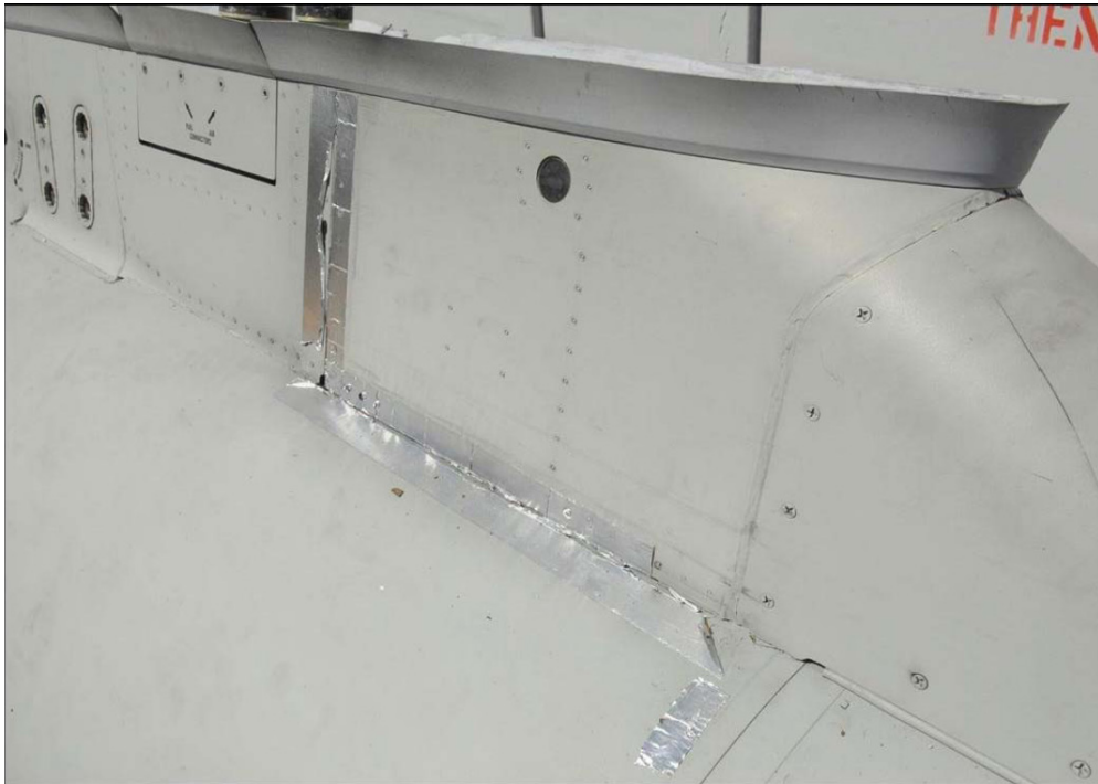
Figure 37: Cracks between tank and integrated pylon and on integrated pylon panels (tried to repair by tape).
